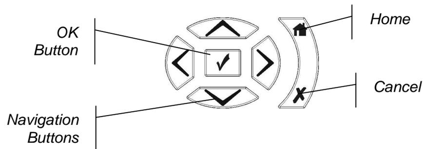
During configuration, the rear illumination of each push button changes, providing a contextual aid to the user. Only those buttons that will do something are backlit. Generally, the up/down buttons are used to cycle through menus and the OK button is used to accept choices.
