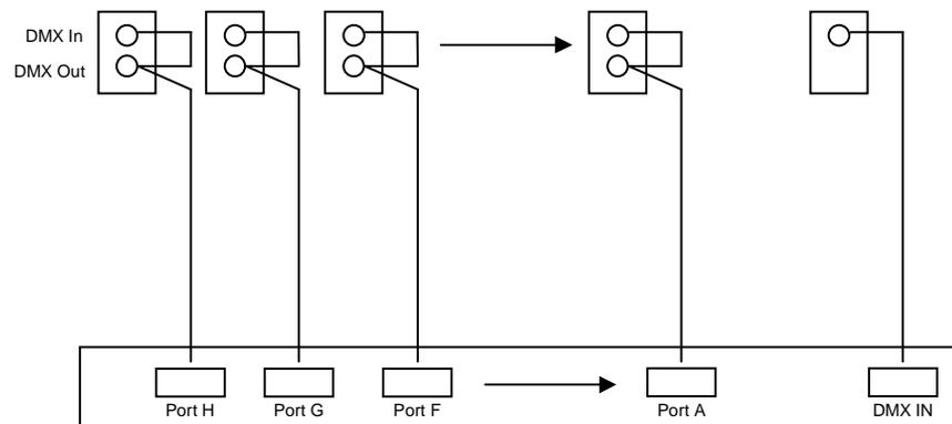
Because RDM-enabled ports can be both DMX inputs and outputs, the *DMX Repeater Pro* is capable of selecting any of the 9 ports on the unit as the splitter's primary DMX input. When in Hub Mode and DMX is not present on any port, the *DMX Repeater Pro* scans each port, listening for DMX. Each port is made an input for about 1/10<sup>th</sup> of a second, while the other ports are disabled.
